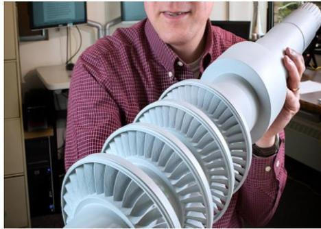
GE Global Research is testing a desk-size turbine that could power a small town of about 10,000 homes. This turbine is not driven by steam it is driven by “supercritical carbon dioxide”. Carbon dioxide in a supercritical state is neither a liquid nor a gas; existing only at very high pressure and temperatures. Don’t let its small size fool you; it can deliver an electrical output ten times larger than steam turbines of comparable size.
