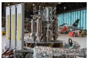
**“KRUSTY experiment successful – ENDED with a 28hr Full Power Test of the nuclear reactor power system called “Kilopower” - the future for space travel.”**
