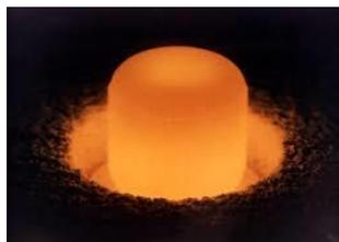
The following is a picture depicting the actual size of the Pu-238 fuel pellet – it is actually the fuel pellet used with the Saturn probe – Cassini.
